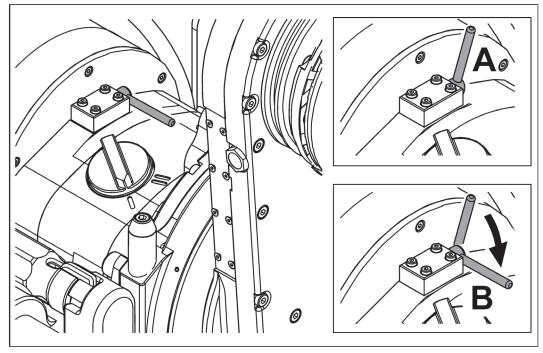
A ⇔ The safety coupling has activated. B ⇔ The safety coupling must be reset by hand.
