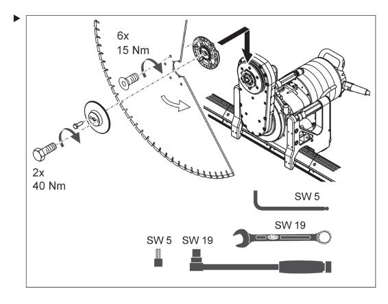
3.4.4 Fixing for normal cuts with saw blades bigger than Ø 1000 mm
